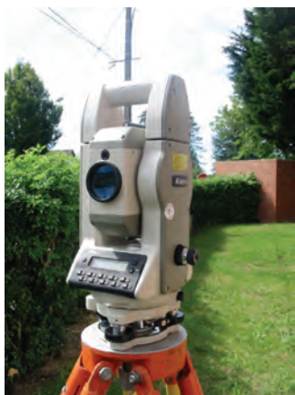
Theodolites are small mounted telescopes that can be moved horizontally and vertically. Navigators and surveyors use them to measure angles and bearings.
