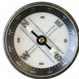
A compass needle points towards magnetic north, which varies by location.
