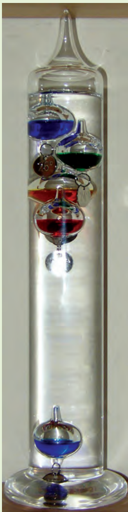
This is a modern-day thermometer based on Galileo's thermoscope.
