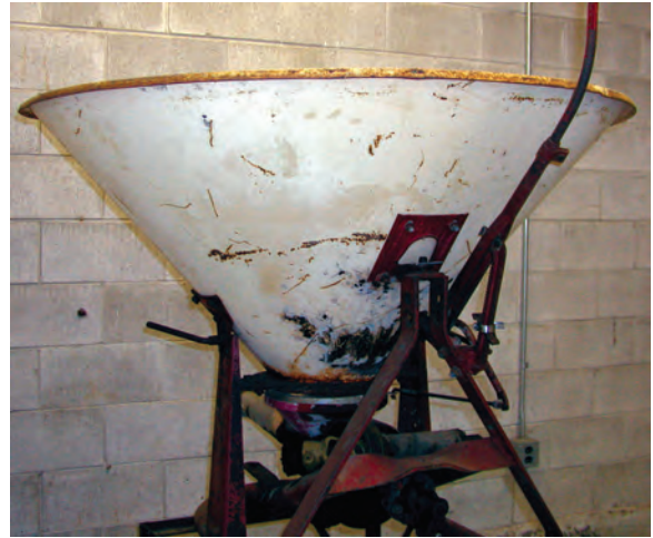
This is an older style hopper made of metal instead of plastic.
