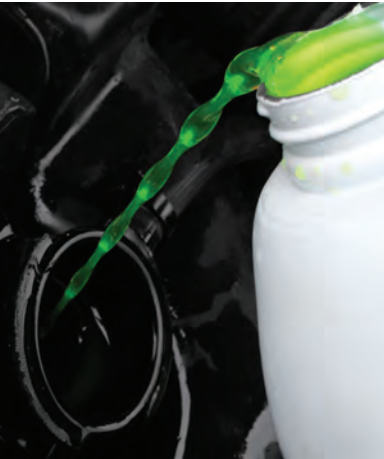
Antifreeze prevents water from freezing and expanding in the cooling system.
