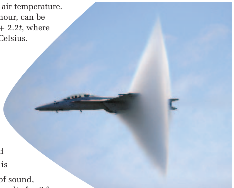
Water vapour created as jet breaks sound barrier
